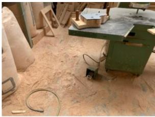
Deposits of wood dust were found in the sawmill and around most of the woodworking machines
