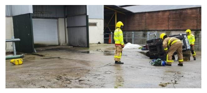
An investigation by the Health and Safety Executive (HSE) found that the areas where FLTs were driven had significant changes in gradient which were not a suitable surface for the type of FLTs in use. The company failed to both identify and control the risk of FLT overturn.
