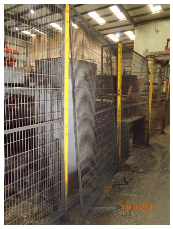
An investigation by the Health and Safety Executive (HSE) found that parts of the perimeter fencing had not been in place since January 2018. The company had also failed to carry out any maintenance necessary to ensure the integrity of the fencing and gates.
