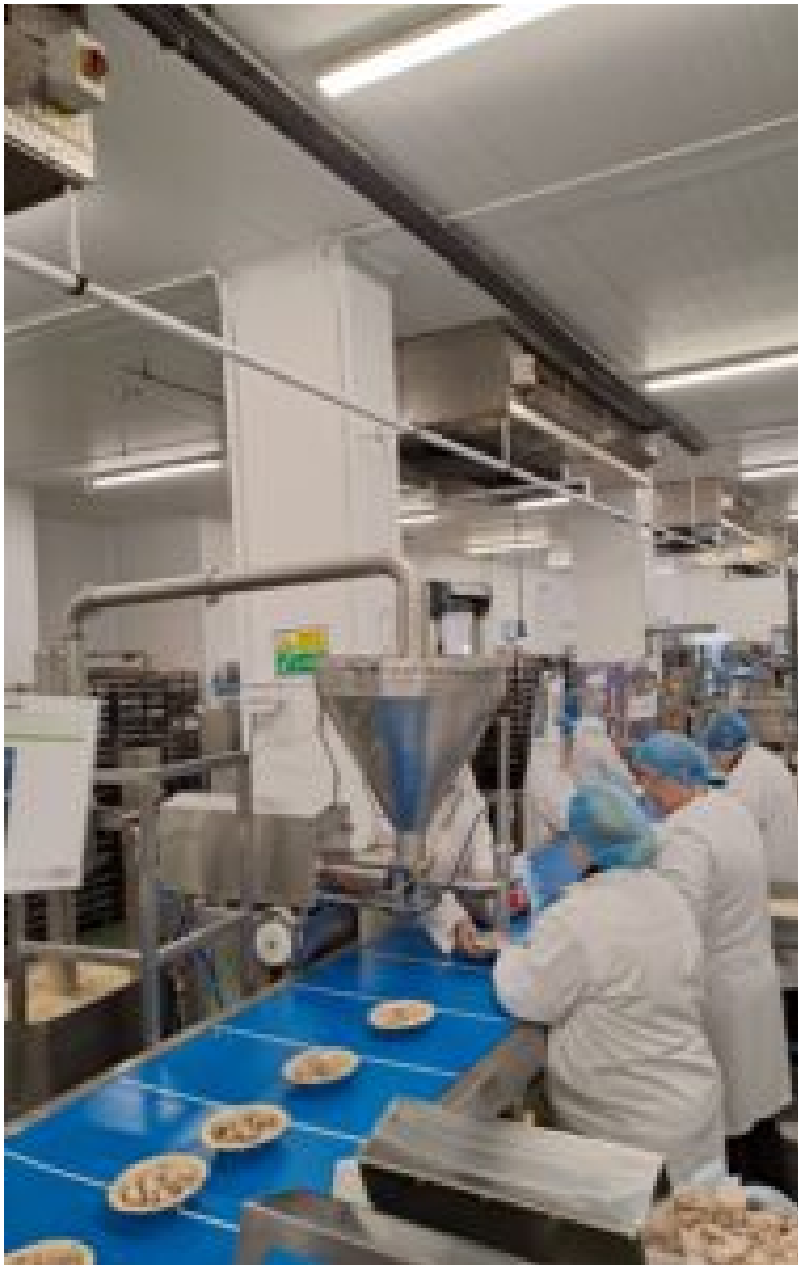
Operators at Cranswick Gourmet Pastry Ltd 'crimping' and weighing pies at the end of the line
