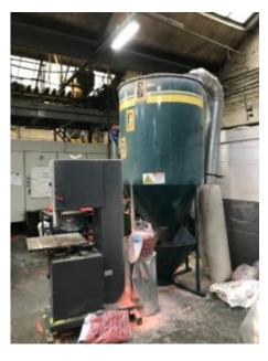
An investigation by the Health and Safety Executive (HSE) found that the blender had not been sufficiently guarded to prevent access to dangerous parts of machinery. There was a large gap of approximately  $4 \times 5$  inches towards the top of the hopper guard. The injured employee had only been operating the machine for one week prior to the incident.
