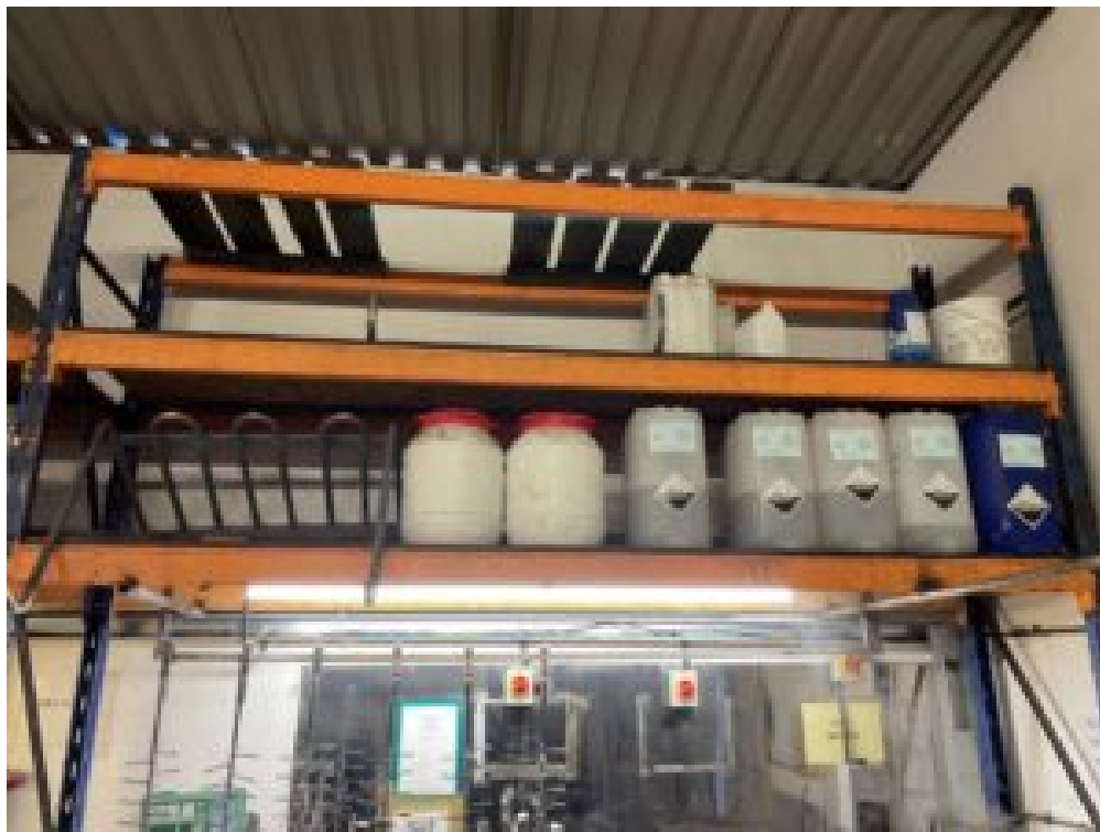
Acids being stored at a high level
