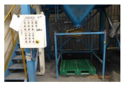
HSE guidance states employers must take effective measures to prevent access to dangerous parts of machinery. This will normally be by fixed guarding but where routine access is needed, interlocked guards (sometimes with guard locking) may be needed to stop the movement of dangerous parts before a person can reach the danger zone. Further guidance can be found here:
