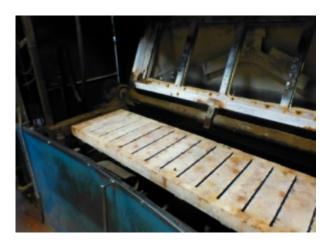
A subsequent investigation by the Health and Safety Executive (HSE) found there was inadequate safeguarding to prevent access between the closing pattern parts of the moulding machine.
