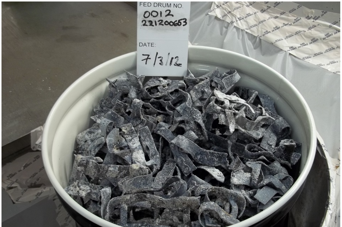
Fuel Element Debris (FED)
