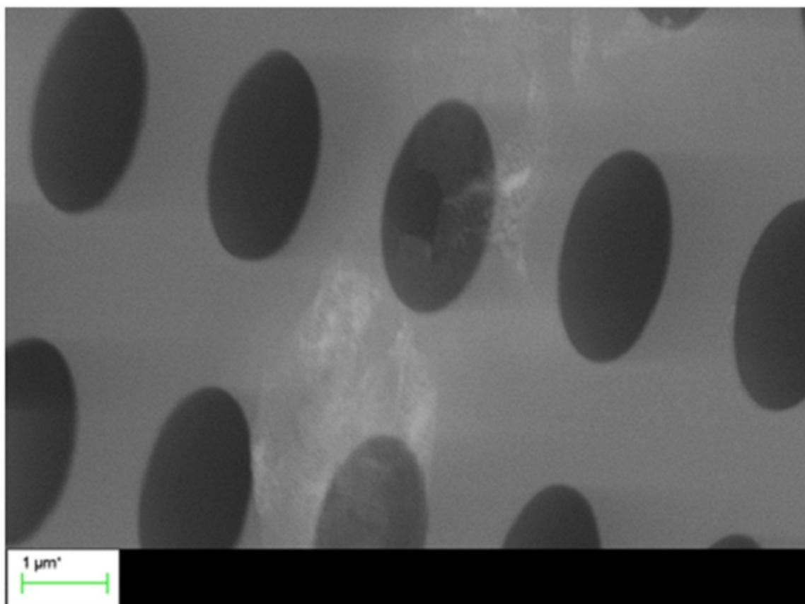
Figure 2: Scanning electron microscopy image of a graphene membrane transferred on a Si<sub>3</sub>N<sub>4</sub> [Courtesy of Professor Sergey Kubatkin, Chalmers University]
