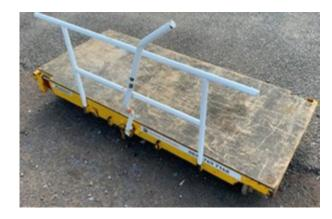
An example of the type of trolley struck by the train (courtesy of Network Rail)
