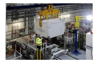
An inactive transport package in the Direct Import Facility
