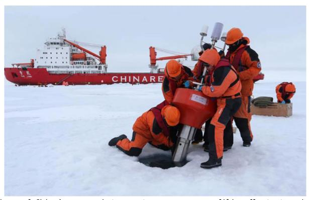
Members of China's research team set up an ocean profiling float at a shortterm data acquisition location near the icebreaker Xuelong, or Snow Dragon, in the Arctic Ocean, Aug 18, 2016. [Photo/Xinhua]
