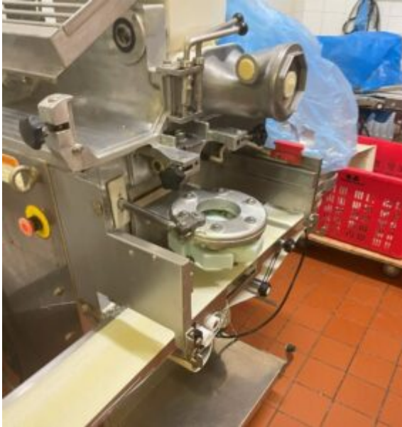
Mochi making machine with missing front guard
