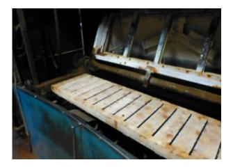
A subsequent investigation by the Health and Safety Executive (HSE) found there was inadequate safeguarding to prevent access between the closing pattern parts of the moulding machine.
