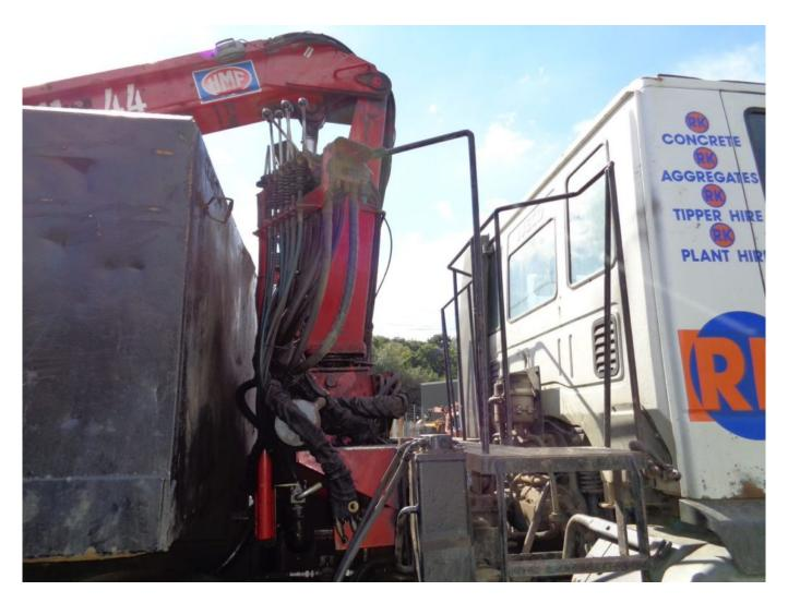
An investigation by the Health and Safety Executive (HSE) found the crane had severe defects, including a disabled safety system, and part of the safety guard around the controls had been cut off, leaving the spike on which his arm was impaled. In addition, the worker had not received appropriate training to operate the lorry loader crane.
