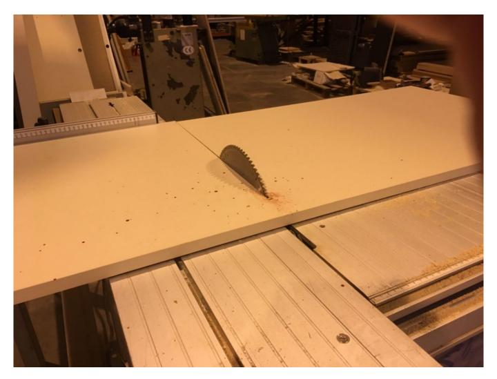
An investigation by the Health and Safety Executive (HSE) found that the worker was pushing the sheets through the saw by hand, without using an appropriate pushstick or jig which would have kept his hand and fingers away from the moving blade. At the time of the incident the crown guard and riving knife were also not fixed to the machine. The investigation also found that there was no Employer's Liability (Compulsory Insurance) policy in place.
