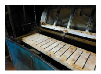
A subsequent investigation by the Health and Safety Executive (HSE) found there was inadequate safeguarding to prevent access between the closing pattern parts of the moulding machine. RSM Castings Limited of Round Spinney Estate North, Portway Close, Round Spinney Northampton, pleaded guilty to breaching Section 11 of the Provision and Use of Work Equipment Regulations 1998 and had been fined £32,000 and ordered to pay costs of £1739.70.
