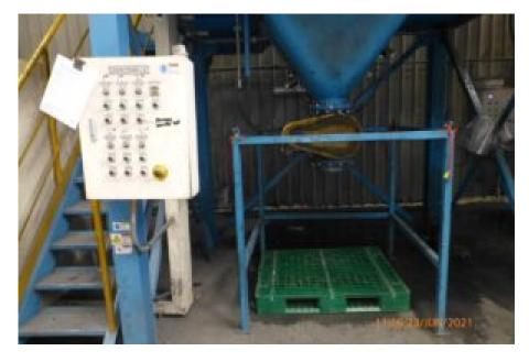
HSE guidance states employers must take effective measures to prevent access to dangerous parts of machinery. This will normally be by fixed guarding but where routine access is needed, interlocked guards (sometimes with guard locking) may be needed to stop the movement of dangerous parts before a person can reach the danger zone. Further guidance can be found here: <u>Provision and Use of Work Equipment Regulations 1998 (PUWER) (hse.gov.uk)</u>
