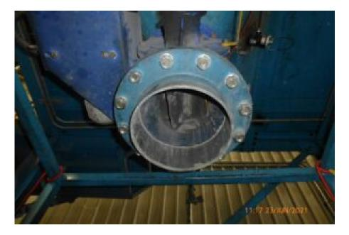
HSE inspector Marcus Pope said: "Every year, a significant proportion of accidents, many of them serious and sometimes fatal, occur as a result of poorly guarded work equipment. In this case this was a wholly avoidable incident, caused by the failure to guard dangerous parts. Had the company added suitable guarding to the outlet of the machine, this life-changing injury would not have occurred."
