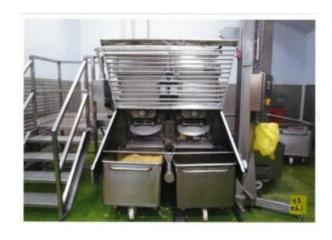
An investigation by the Health and Safety Executive (HSE) found that the machine continued to run when the safety guard was lifted and failed to respond when the emergency stop was pressed. The interlocking system was inadequate, and the company had failed to ensure that the machine was effectively maintained. These matters were exacerbated by poor communication between the shop floor and maintenance and an inadequate fault reporting system.
