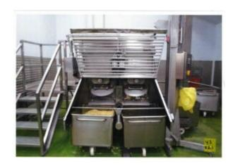
An investigation by the Health and Safety Executive (HSE) found that the machine continued to run when the safety guard was lifted and failed to respond when the emergency stop was pressed. The interlocking system was inadequate, and the company had failed to ensure that the machine was effectively maintained. These matters were exacerbated by poor communication between the shop floor and maintenance and an inadequate fault reporting system.
