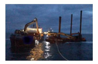
Our investigation report into the immobilisation of the dredger Shearwater, after its propeller shafts were fouled by its own towline while towing the barge Agem One on 9 April 2020, is now published. Shearwater was damaged and holed, resulting in flooding, after repeatedly colliding with the unmanned barge during the accident.
