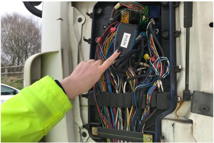
DVSA examiners will be checking lorries for emissions cheat devices, such as the AdBlue emulator seen attached to this vehicle.
