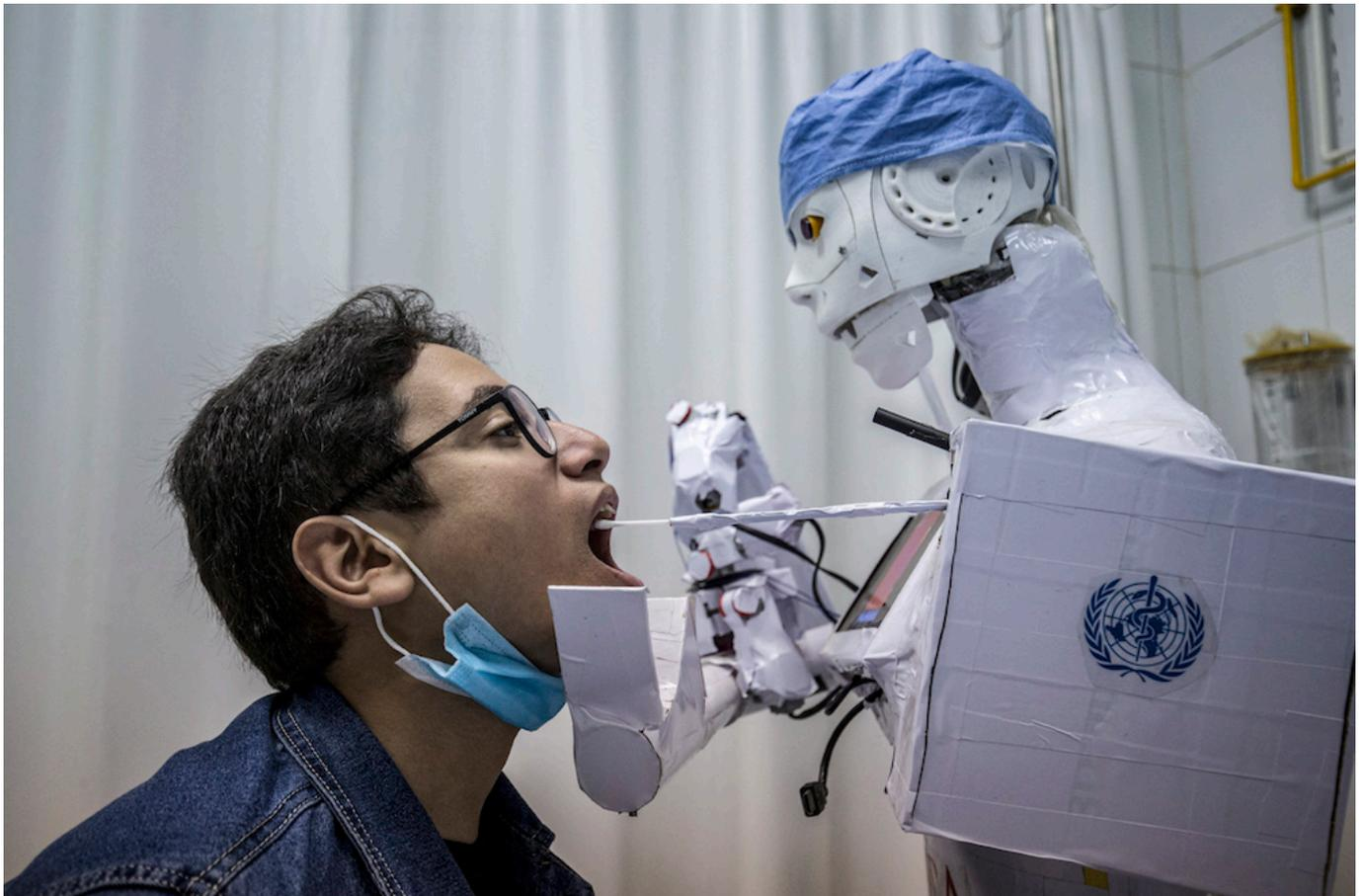
A prong extending from the CIRA-03 remote-controlled robot prototype approaches the mouth of a volunteer to extract a throat swab sample, as part of a self-funded project to assist physicians in running tests on suspected COVID-19 coronavirus patients in a bid to limit human exposure to disease-carriers, at a private hospital in Egypt's Nile delta city of Tanta. (AFP/File Photo)
