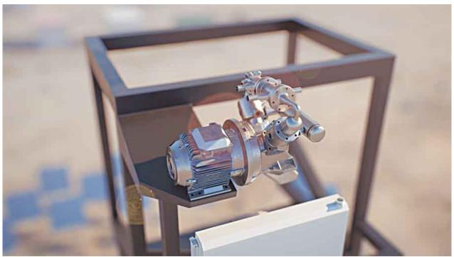
The Stirling engine efficiently converts thermal energy into mechanical movement to generate electricity. (Supplied)
