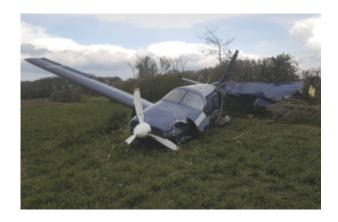
During an experimental flight near Cranfield Airport of a modified Piper PA-46-350P (G-HYZA), an electrically powered aircraft with electrical power from hydrogen fuel cells, suffered a loss of power to the electrical motors. This meant a forced landing was carried out, which severely damaged the aircraft, the crew were unharmed.
