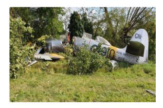
During the second flight of Hawker Sea Fury T MK.20 (G-INVN) following maintenance, the engine oil temperature rose and the oil pressure started to fluctuate. The engine then seized, forcing the pilot to make a landing in a field. The aircraft was extensively damaged and both occupants suffered serious injuries.
