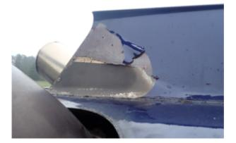
Whilst hovering at 20 ft above ground level, smoke was observed coming from the engine exhaust of an Airbus Helicopters AS355 F1. The pilot was informed and the helicopter landed immediately. After landing a fire was also observed, a fire warning subsequently illuminated, and the pilot activated the fire extinguishing system. The pilot completed the shutdown checks and exited the helicopter. There were no injuries.
