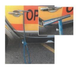
An Embraer 145 landing at London Southend Airport ran over a general aviation towbar which had been dropped on the runway. No damage was caused to the aircraft.
