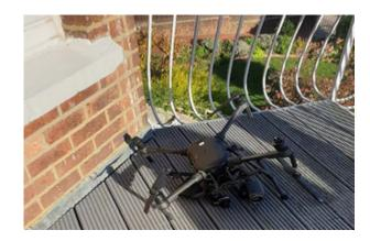
A DJI Matrice M210 Version 1, quadcopter unmanned aircraft (UA) was being flown during a police operation when the wind at 400 ft exceeded the forecast wind, the manufacturer's wind limit and the maximum restricted speed of the UA. The UA drifted beyond visual line of sight and then communication with it was lost. When the battery level was low it entered an auto-land mode but collided with the wall of a house, damaging its propeller blades before coming to rest on a balcony.
