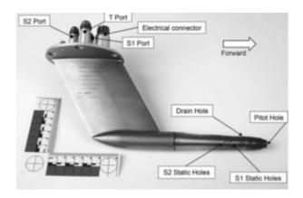
While climbing to 19,000 feet, the pilots received an 'altitude mismatch' message and returned to Exeter Airport. An inspection after landing found a small white crystalline deposit covering three of the four static pressure holes on the left primary static probe. Primary static probes are used to measure pressure, which along with other data allows the Air Data Units to calculate parameters such as altitude, indicated and true airspeed and temperature.
