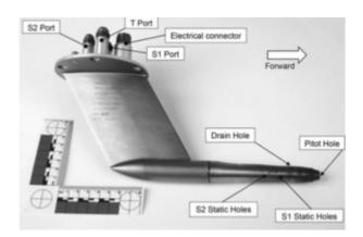
While climbing to 19,000 feet, the pilots received an 'altitude mismatch' message and returned to Exeter Airport. An inspection after landing found a small white crystalline deposit covering three of the four static pressure holes on the left primary static probe. Primary static probes are used to measure pressure, which along with other data allows the Air Data Units to calculate parameters such as altitude, indicated and true airspeed and temperature.
