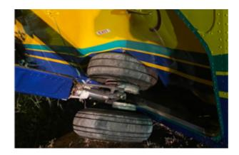
On landing, the pilot was unable to maintain directional control and reported the left brake was 'spongy'. The aircraft veered off the right side of the runway and impacted the bank of an adjacent drainage ditch. One passenger suffered minor injuries as a result.
