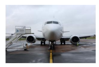
During an approach at Exeter Airport, the aircraft became unstable after the point where the crew had declared the approach stable and continued. During the final 500 ft the rate of descent exceeded the required 500 ft stable approach criteria on four occasions. All bar the first of these excursions were accompanied by GPWS "SINK RATE" alert. The subsequent hard landing resulted in extensive damage to the aircraft. There were no injuries.
