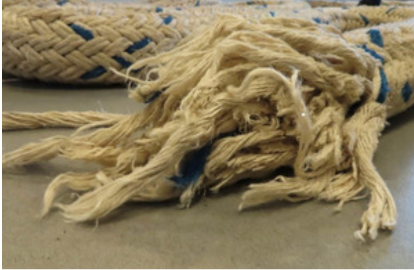
Parted mooring line
