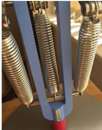
The springs on a Type 75 Anglepoise lamp
